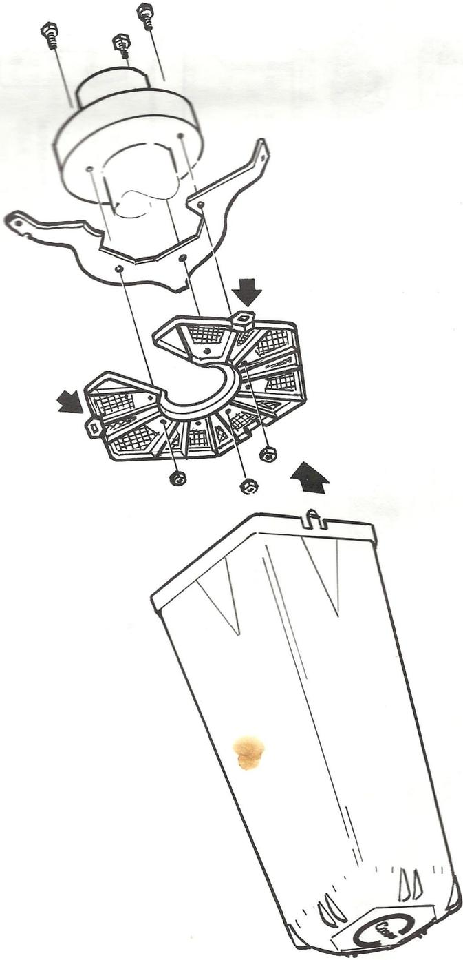
**Note:** Place feedhorn cover over the LNA feedhorn and press plastic base near each tab to lock.
