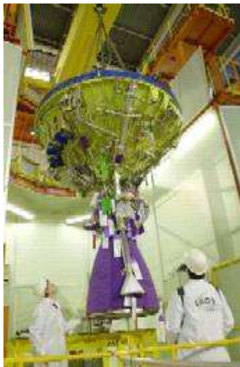
ESC-A thrust frame © Airbus Defence and Space
