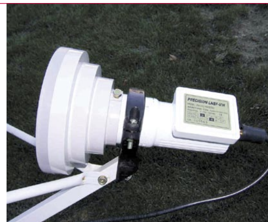
Astrotel LNB with Cone-shaped Scalar Ring on the 1.0-Meter Dish |
