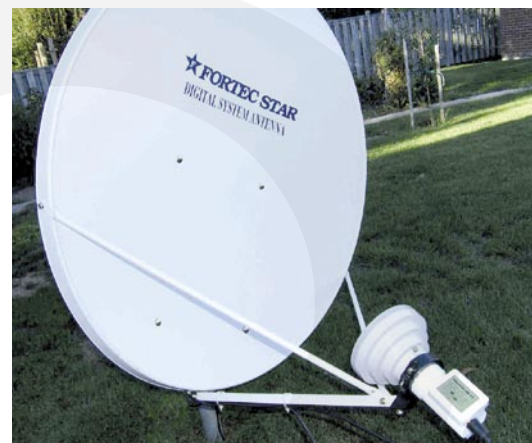
The Complete 1.0-Meter Dish Assembly |
