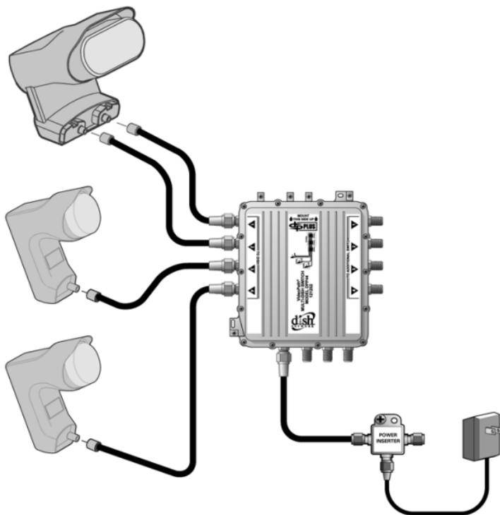
**Figure 6. DISH Pro Plus 44 Connections**
