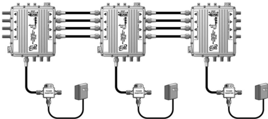
**Figure 7. Additional DISH Pro Plus 44 Switches**
