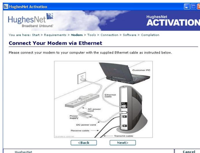
3. After the activation software confirms the customer's PC meets the minimum requirements, proceed with antenna installation, cabling, and commissioning. Installers must use their laptops to commission the system, not the customer's PC. **Do not connect the HN7000 to the customer's PC until directed to do so by the HughesNet Activation CD.**
