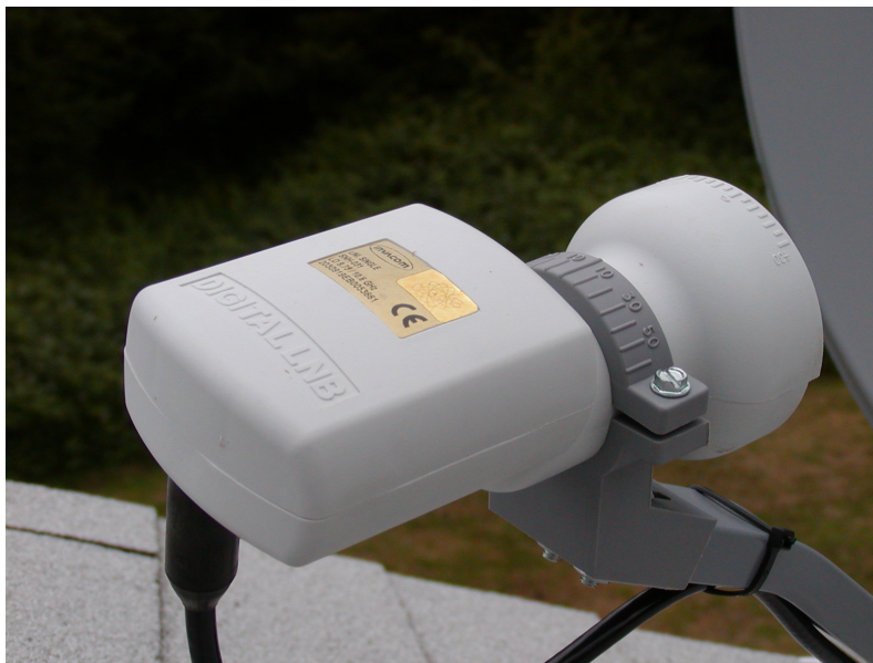
LNBF Set to 12 O'clock Position
