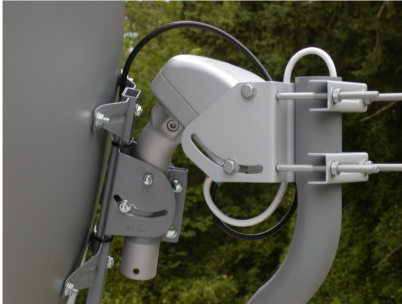
Carefully Route and Secure Coax Cables
