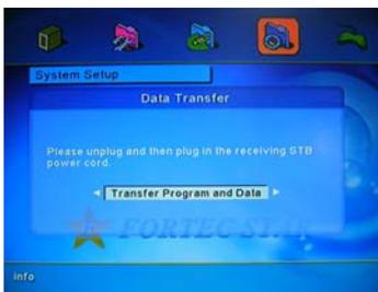
All program and / or data in the master receiver can be transferred to the next(slave) receiver using this function.
