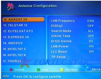
This mode will display the Antenna adjustment menu on the screen and can adjust all required installation information for each selected Satellite.
