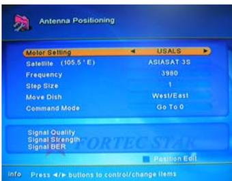
This mode will allow you to use a DiSEqC1.3/2.3 motor controlled by USALS (Universal Satellite Automatic Location System).
