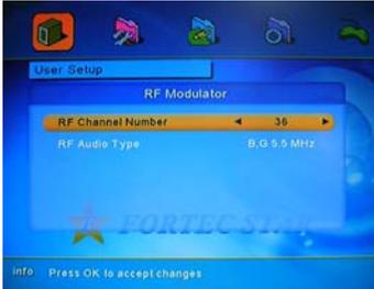
If receiver is connected to the TV by an RF lead, you can select the RF modulator channel and RF audio type. Channel 36 is the default factory setting for the channel to which your TV must be set in order to view the output of your receiver. If this channel is currently being used as a broadcast channel or if you are getting interference on this channel, you may
