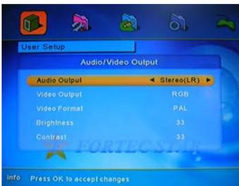
You can select which type of audio and your receiver for audio outputs video : you can select one of various stereo outputs or mono sound. For video output, you may choose between RGB and and CVBS. If your television set is a Multi-System TV capable of displaying either PAL or NTSC, then you may set the Video Format to Auto, If not, set the Video Format to either NTSC
