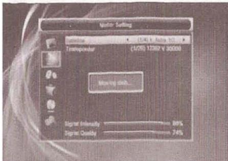
Switching the satellite can move the dish to the right place.
