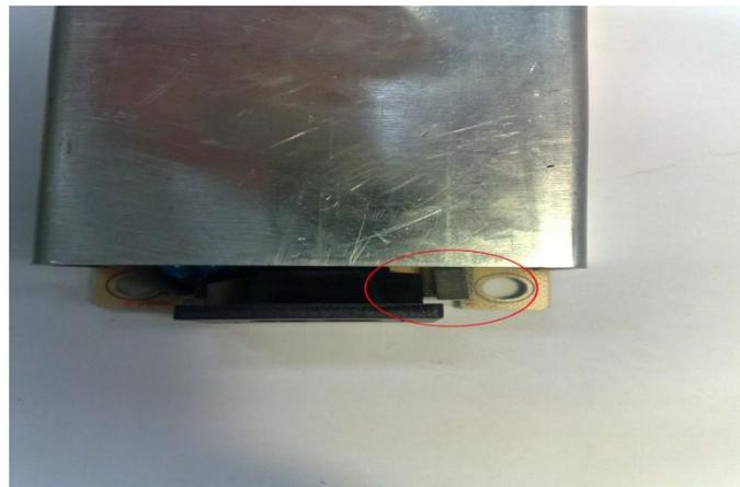
1.3. Test the continuity on the pins of the diode bridge (BD1).
