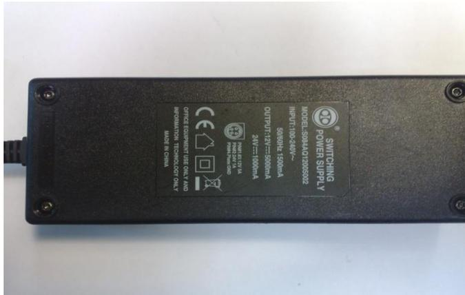
1.2. Unscrew, and remove pcb board from inside. Locate and replace fuse (F1).
