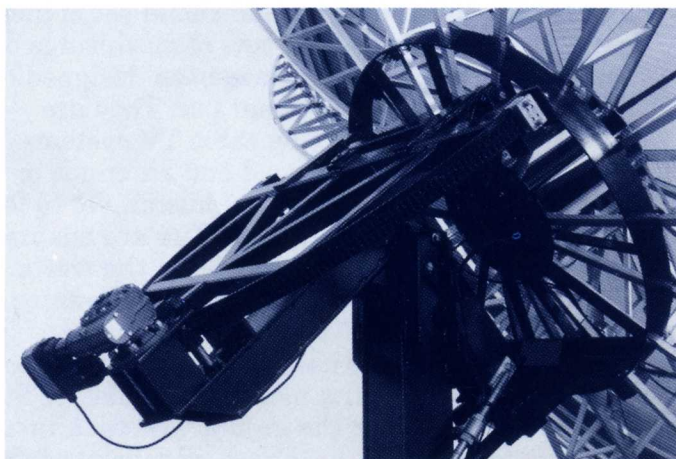
This view of the T24 mount shows the trusses, spool, hub ring, chain driven D ring, D ring drive motor and elevation beam.
