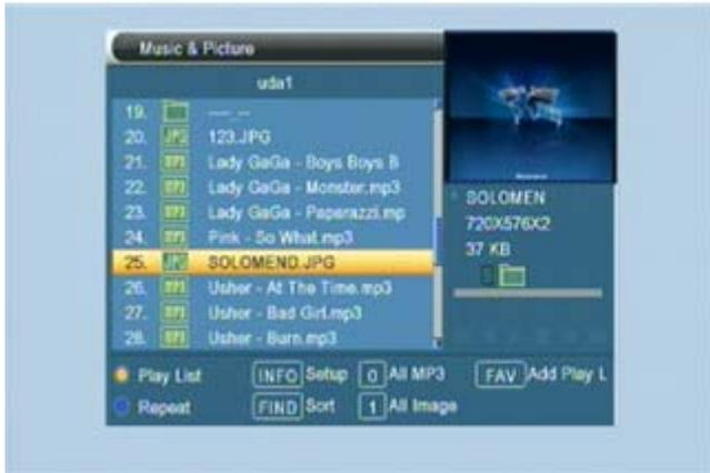
You can preview the picture at the top right corner if the scroll bar is on the picture files (JPG, BMP), and show the logo when at MP3 file. Move scroll bar when press up/down key, page up or down by page key. Go into sub-directory when press ok key in the file directory, play the selected file when scroll bar is on the file, automatic return Music&Picture menu after play is over.
