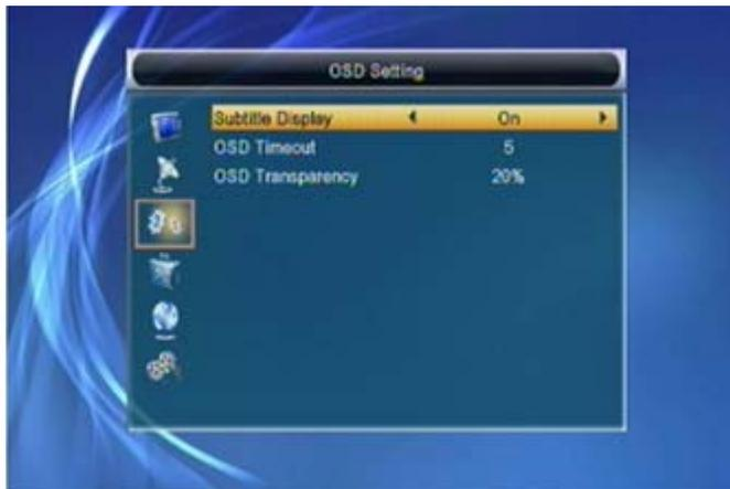
1 OSD Timeout: When you switch channels in full screen, there will show up some information about current channel on the lower of the screen. And regarding to the duration of these information show up on the screen, you can press [Volume Up/Volume Down] key to set the time. The range of the duration is "1 second ~ 10 seconds".
