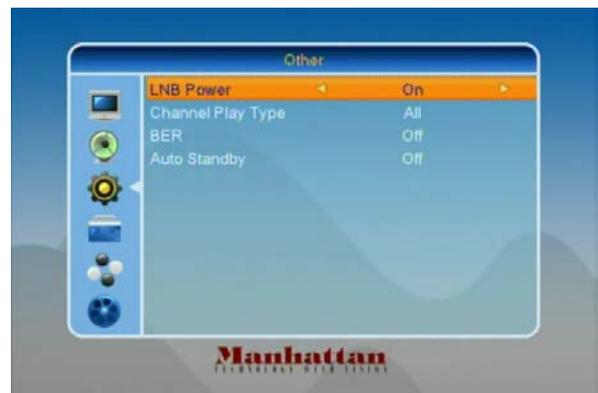
**LNB Power:** You can set this option to “On” or “Off”. If the setting is set to “On” the receiver will supply power to the satellite antenna. “Off” will not supply power to the antenna.
