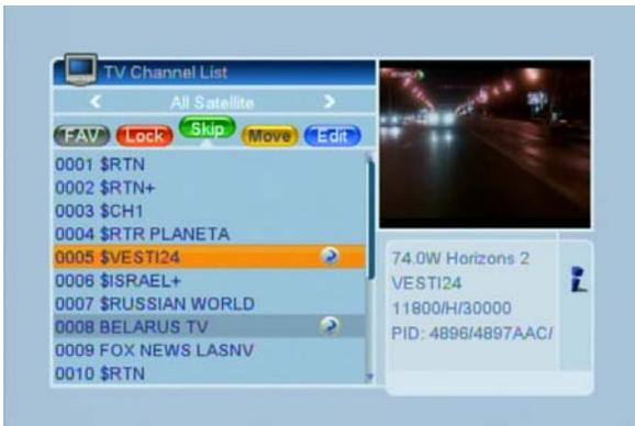
You can move the highlight using [Up/Down] and [OK] to make a skip mark on the right side of the channel. After you save and exit the menu, the channel will be skipped when change channels in full screen.
