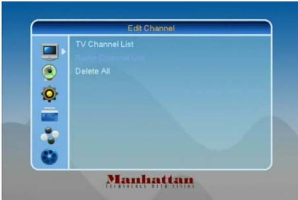
Use the [Up/Down] keys to switch between the menu pages “Edit Channel, Installation, System Setup, Tools, and Game, and Record”. Press [OK] or [Right] to enter “Edit Channel”. If menu lock is on, it will display a dialogue for the user to key in password. The default password is “0000”.
