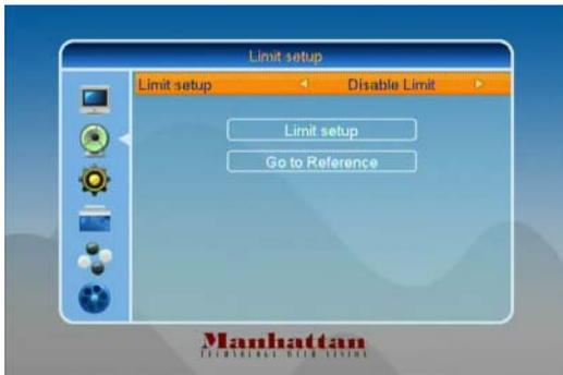
When you set "Limit Setup" to "West Limit/East Limit", you can move the highlight to "Limit Setup" Line and move the dish to east or west by pressing [Left/Right] keys manually. When you are moving the target place, press [OK] key to save the point.
