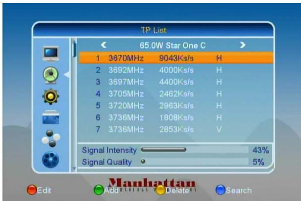
Use the [Left/Right] keys to switch satellite. Press the [Red] key to open “Edit TP” menu. User can edit TP info. Frequency: “3000~13450 MHz”, Symbol Rate: “1000~45000Ks/s”.
