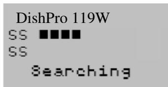
When you are close to the optimal position, the second bar will show finer data that allows perfect alignment.
