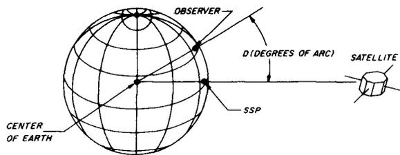
fig. 2. The observer's position on the earth's surface, in relation to the imaginary straight line shown in fig. 1, yields the angle  $D$ , which is used to calculate antenna elevation angle as discussed in the text.
