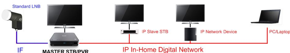
The master STB often features the possibility of recording content. This document does not specify how recorded content is accessed nor how content scheduling is handled. Such use cases are described in the DLNA protocol specifications. The SAT>IP protocol purely describes access to live media content.
