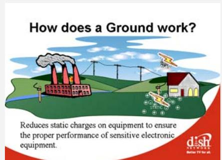
Because the problem only occurs when the antenna discharges static electricity, the technician normally can not identify the cause while on site. Typically the technician will RA the receiver or LNBF. Did this solve the problem? Will this customer have the same complaint again? Do you think this customer will churn due to his/her frustrations? With a proper ground, the static is sent into the ground before it can build up and cause an issue."
