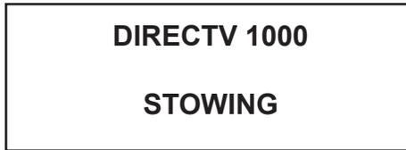
The unit will stop what it is doing and begin to return to the stowed position. The TRAV'LER Interface WILL NOT TURN OFF unless the TRAV'LER mount is successfully stowed.
