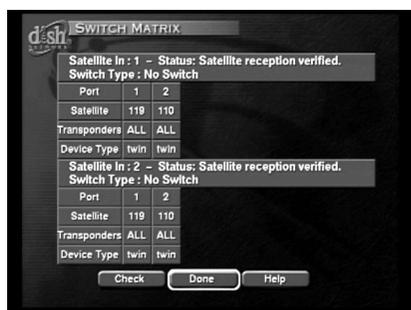
This time, you *must* see that you have signals from both the **110 West** and **119 West** Satellites *for both* **Satellite In 1** and **Satellite In 2**, and the message “Satellite reception verified” for both satellite inputs. Select **Done** to exit this menu.
