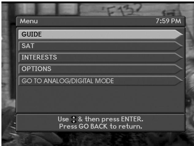
Only option 5, "Go to Analog Mode" is unique to the front panel controls. All other screens are identical to the screens accessible via the remote control. Option 5 allows you to view the output of your analog receiver without changing the current settings of the Digital Sidecar. To revert to the digital picture mode from the front panel while in the analog mode, press the Menu key.
