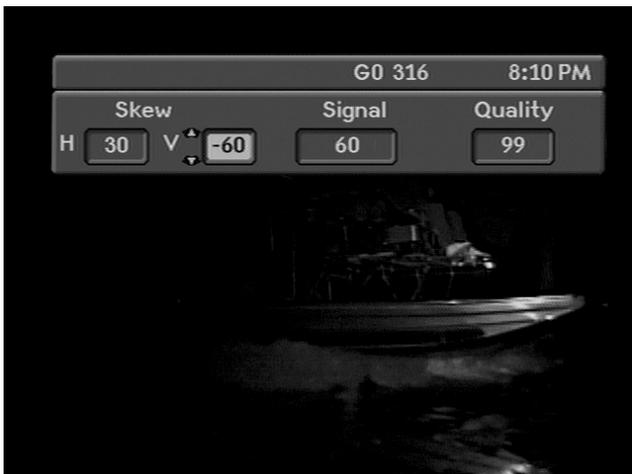
Adjust the SKEW to peak the Signal and Quality levels. You may also need to “bump” the dish east or west using your analog receiver to maximize the signal. If you are unable to receive an acceptable signal level and quality using an LNBF, you may need to switch the feedhorn setting to a rotation of 90°. See page 54 for more information about this feature.
