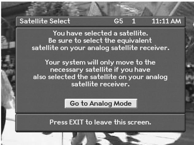
If you press ENTER your Digital Sidecar will select analog mode and enable viewing of your analog receiver video output. You will need to utilize the analog receiver remote control to select the equivalent satellite to move your satellite dish to the proper location. After the satellite dish has moved, utilize the blue A/D key on the Digital Sidecar remote control to resume digital program viewing.
