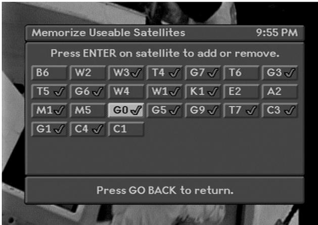
Press EXIT. Select 9 on your remote control. Press ENTER; this selects G0-9. This will change your receiver to the channel 9 to receive digital information. Check to see if the satellite icon on the front panel is green. If not, you may need to adjust your position or skew settings on your satellite dish.
