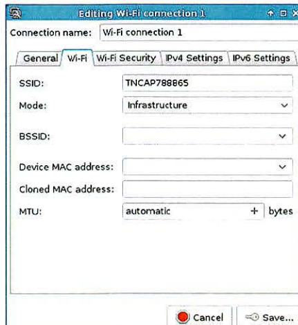
FIGURE 3: Pidora Wi-Fi configuration panel.
