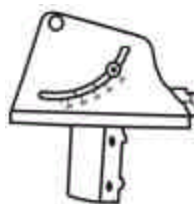
AZ/EL Mount/Mast Clamp Assy
