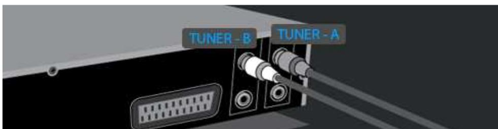
In this configuration you receive exactly the same satellites with the same antennas configuration but on 2 separated cables. For example you have a Monoblock LNB with multiple exits, or you have an external DiseqC switch with multiple exits.
