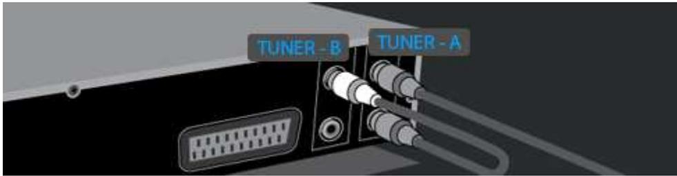
In this configuration you have only one cable that come from your LNB (Antenna) to your Azbox and you loop through both tuner (Out of tuner-A is connected to In of Tuner-B). In this setup, the Azbox handles both tuners (so you don't have to care about tuner-A or B) but it has disadvantages.
