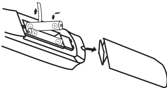
⇒ Insert two batteries into the battery compartment - paying attention to the indicated polarities and push the cover of the battery compartment carefully until it is locked.
