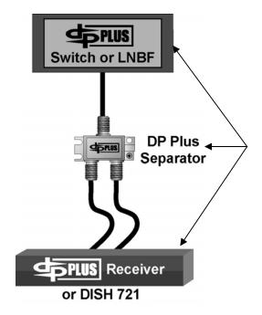
For the single-cable dual-tuner advantage, all three components must be DISH Pro Plus.
