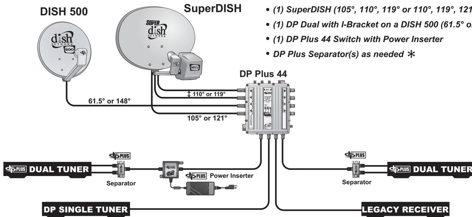
Each DP Plus 44 Switch requires a Power Inserter on port 1
