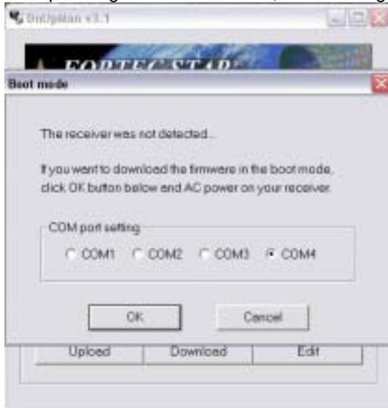
5. When you see the message "Waiting for the response of your receiver", turn on the power switch located in the back of the receiver.
