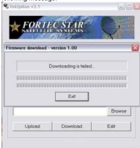
Even though the software has successfully downloaded, the "failed" message appears. This is due to the fact that the new software has changed the communication function of the RS232 port on the receiver. The Loader does not get back the expected return message from the RS232 port that it gets from downloading a normal file.
