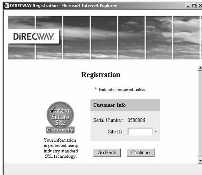
Figure 51: Registering a remote terminal: entering the site ID
