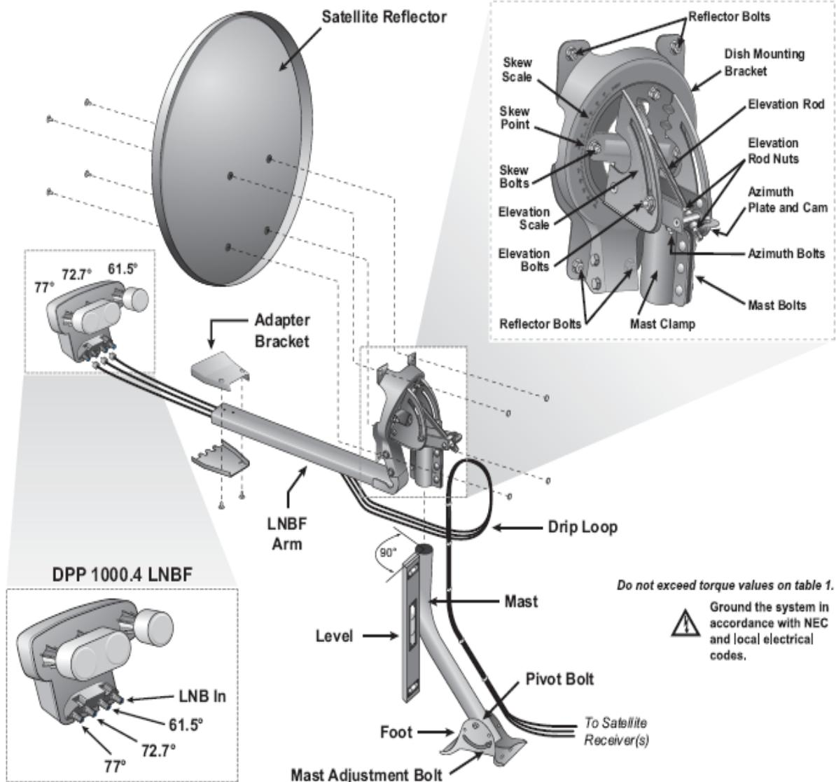
The Dish Pro Plus 1000.4 dish kit and LNB are very similar in function to the Dish Pro Plus 1000.2 dish kit and LNB. Both support the use of the DPP separator, provide 3 primary orbital locations, and support the use of a Wing Dish for an optional fourth orbital location. Both are also not to be combined with a switch of any kind.
