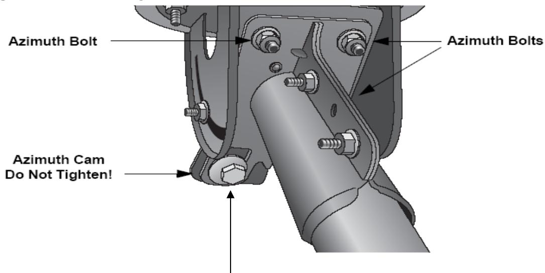
Loosen all 3 bolts and maximize the signal, then re-tighten all 3 bolts, but do not torque the Azimuth cam. The azimuth can be adjusted up to 3 degrees in either direction. Adjustments greater than 3 degrees will require loosening the mast clamp bolts. Check for signal strength from the remaining orbital locations after fine-tuning is complete.
