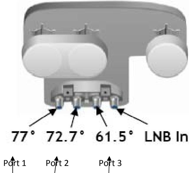
Dish Network recommends “rough peaking” the reflector on the  $72.7^\circ$  signal which is brought in by port #2 on the LNB. Once the dish has been “rough peaked”, use the fine-tuning adjustments for azimuth and elevation to maximize the signal.
