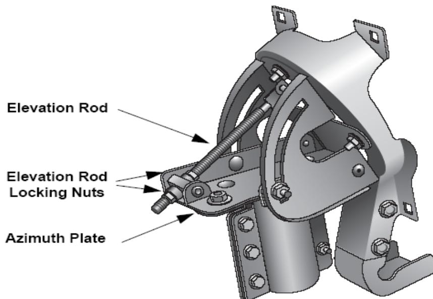
Loosen the elevation nuts and adjust the elevation to achieve maximum signal. Then tighten the top elevation nut, followed by the remaining elevation nuts.
