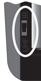
Figure 3: UHF Pro/IR switch inside 21.0 battery compartment
