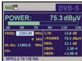
Signal measurement on RAI transponder on HOTBIRD 13° east. Conventional single LNB (left) and Global Invacom optical LNB (right)
