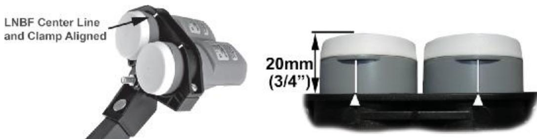
Install two GEOSATpro Mini Bullet LNBFs into the Twin LNBF Clamp, align the centering line on the top of each LNBF with the centering pointer on the clamp. Slide the LNBF forward towards the reflector so the front face of the LNBF is 20mm (3/4") offset forward of the clamp. Securely tighten both clamp screws (2).
