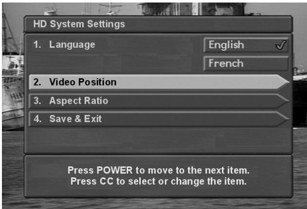
To scroll through the list of options, use the POWER button on the front panel. To make a selection or change an item, press the CC button. For example, if you wish to change the language setting to French, press Power once, then press the CC button to select the French language option. Press POWER to move to "Save & Exit" which will exit the menu and return to television viewing.
