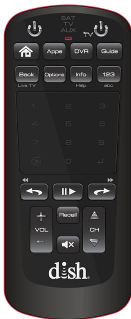
If the missing remote control is paired to this Hopper 3 receiver and within radio frequency (RF) range, there should be a series of tones you hear to help find the location of the remote. It may take up to 30 seconds after touching LOCATE REMOTE before you hear the tones. Press any button on the remote to turn off the Locate tones after finding the remote.
