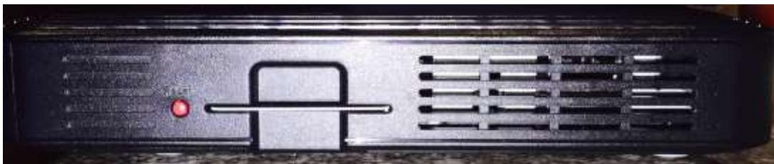
The access card is now on the right side of the unit along with the red button for rebooting the unit. This is similar to other models.
