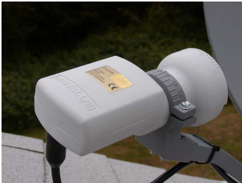
LNB Set to 12 O'clock Position
