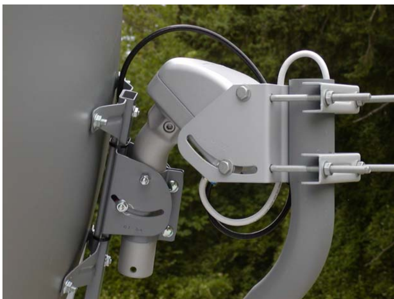
Carefully Route and Secure Coax Cables
