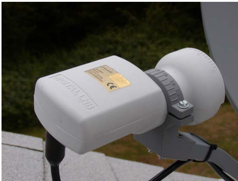
LNB Set to 12 O'clock Position
