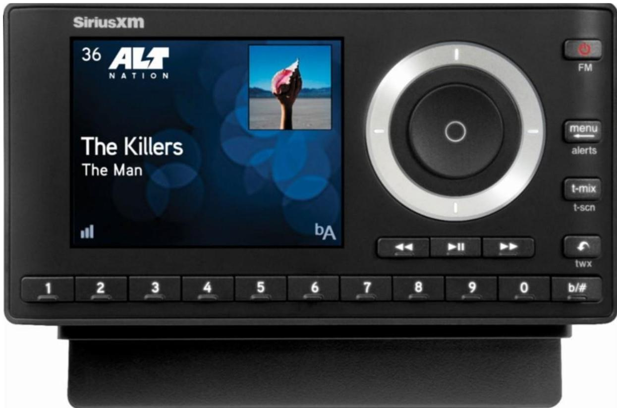
**Optional and Mandatory Equipment Needed.** If you are connecting the Onyx Plus with an audio cable, you need a ground loop isolator: <https://www.amazon.com/Mpow-Ground-Isolator-Stereo-System/dp/B019393MV2> Without it, the noise level on the receiver is fairly high. With it, the sound is excellent. I stuck mine behind the bracket using high strength Velcro.
