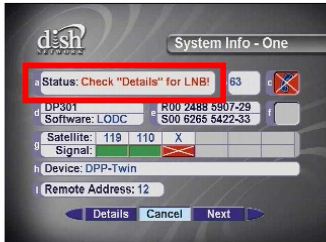
If this Field's Status says "**Check 'Details' for LNB!**", select the onscreen "**Details**" button to view the details of the signal scan.
