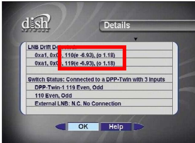
If any of the LNB Drift values are equal to or greater than +/- 5.00, **REPLACE** the LNBF to prevent a possible future Trouble Call.
