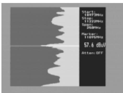
Rotate the LNB so that either the Horizontal or Vertical polarisation will be in its maximum position –adjusting the **cross-polarisation**.
