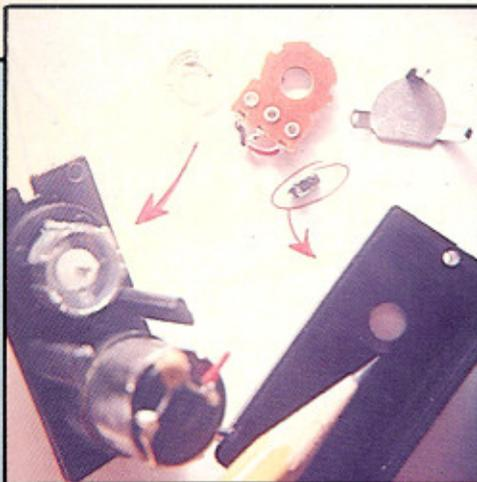
Solder two leads to motor contact. ▶
