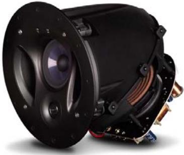
Off-axis listening is also greatly improved through the Vanishing Series in-ceiling models. The woofer is mounted to the rear of the enclosure; while the mid- and high-frequency drive units are mounted to the front baffle. Since the smaller, less directional front drivers are dedicated to only reproducing midrange and high range, they inherently offer more even frequency response to listeners sitting on or off axis in a home theater environment.
