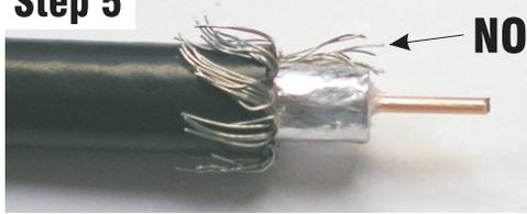
Fold the small 'drain' wires back over the PVC jacket. Inspect the wires carefully to insure **all** wires are folded back neatly.
