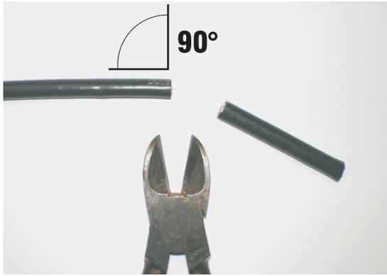
Cut the end of the RG-6 cable cleanly with sharp cutters at a 90° angle.
