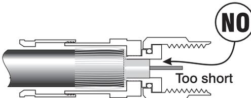
Continue pushing and twisting until the white dielectric foam is flush with the inside face of the connector.
