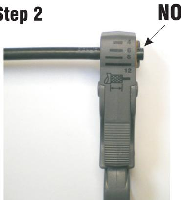
Insert the RG-6 coax into the wire stripper so the end of the coax wire is flush with the side of the wire strip tool.
