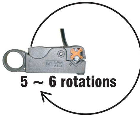
Turn the wire strip tool five or six full and continuous revolutions around the coax wire.
