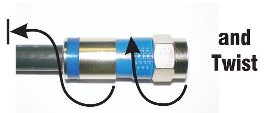
Gently fit the PV-6 RidgeLoc™ connector onto the coax cable. Insure the connector slides over the top of the aluminum foil layer. Press the fitting onto the coax with side-to-side motion
