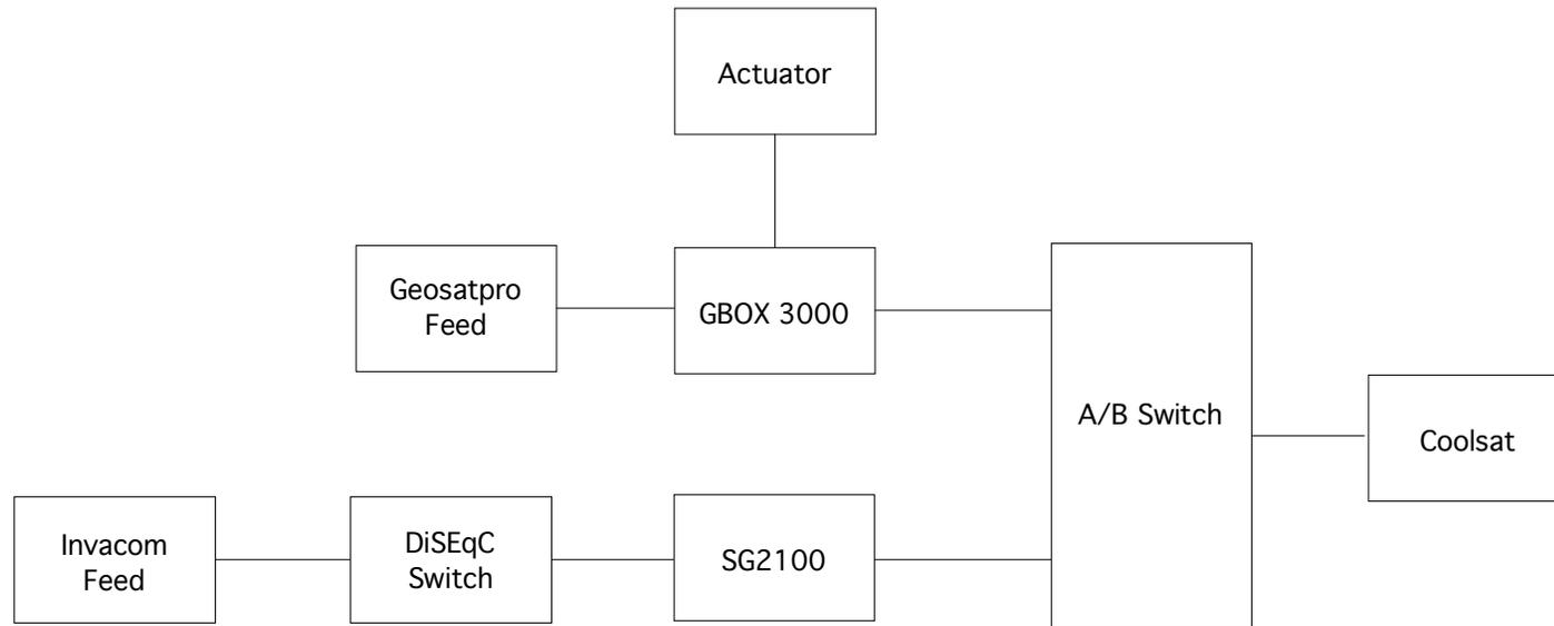
Note: there are automatic switching mechanisms that could eliminate the A/B manual switch.
