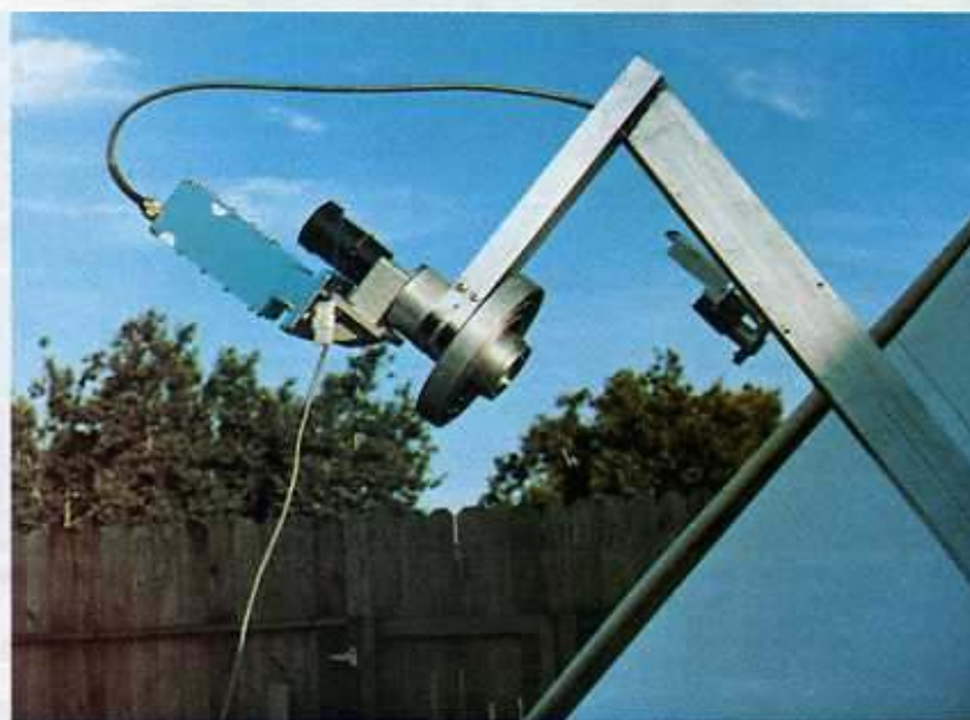
Chaparral .3F/D Feed On Antenna. Note Adapter Ring
