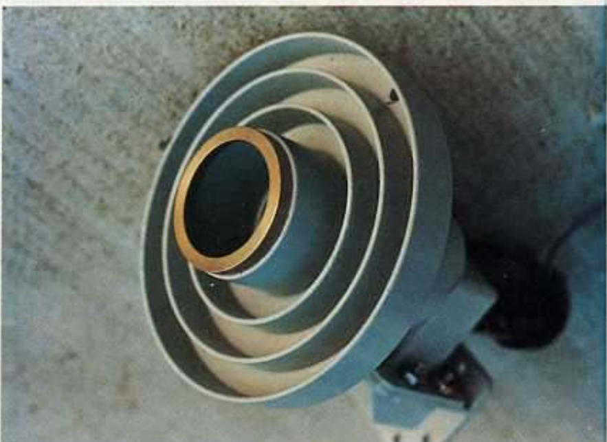
Chaparral Polarotor II with .3 F/D Ring Installed.
