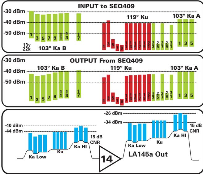
Model SEQ409 is used to reduce the lower Ka signal levels to obtain the maximum un-distorted output from model LA145a amplifier.
