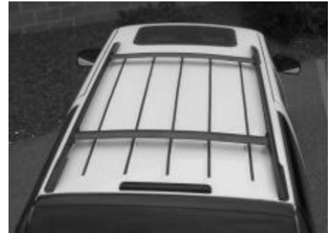
Figure 28: "Skid Ribs" and brakelight
