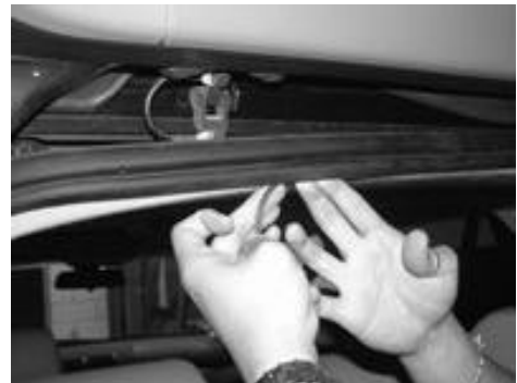
Figure 29: Cable routed through roof end and tailgate under the rubber molding
