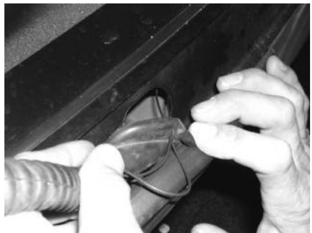
Figure 15: Entering the trunk through cable channel
