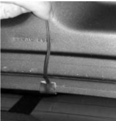
Figure 22: Routing the cables around the trunk lid rim
