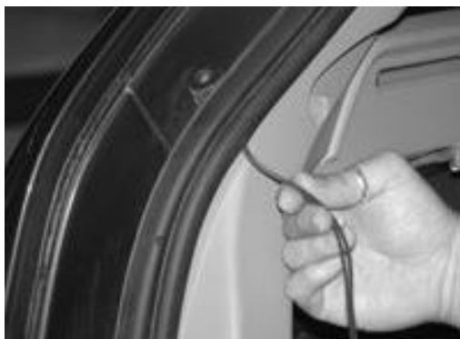
Figure 30: Hiding the cable under the rubber molding
