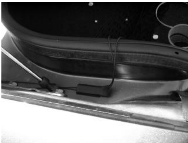
Figure 17: Cable routing along the trunk rubber molding
