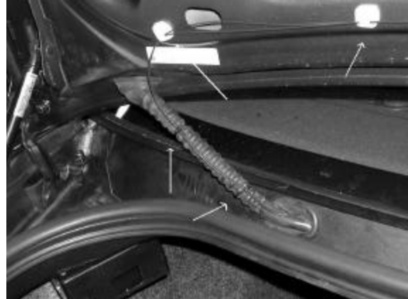
Figure 23: Attaching the cable to the cable channel
