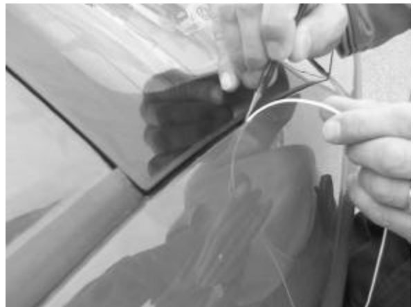
Figure 14: Lifting up difficult molding for routing each cable in both directions
