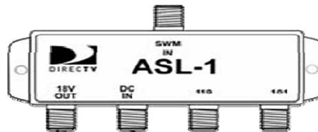
If an ASL is not available then a single port power passing two way splitter (rated @ 2MHz - 2150MHz) can be used **ONLY** with the BirDog and Super Buddy meters.
