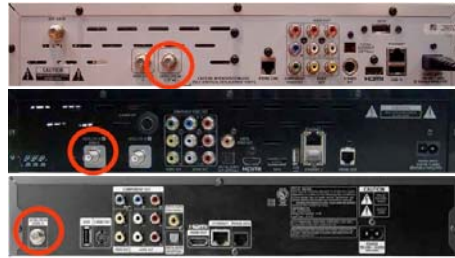
Figure 5 SWM Port on HR20, HR21, and H21 (from DirecTV Install Presentation)
