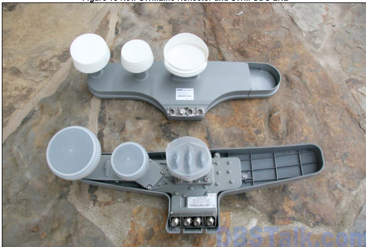
Figure 14 Direct Comparison between the two LNBs; Note the 4 Ports versus 1 Port Only on the SWM ODU LNB
