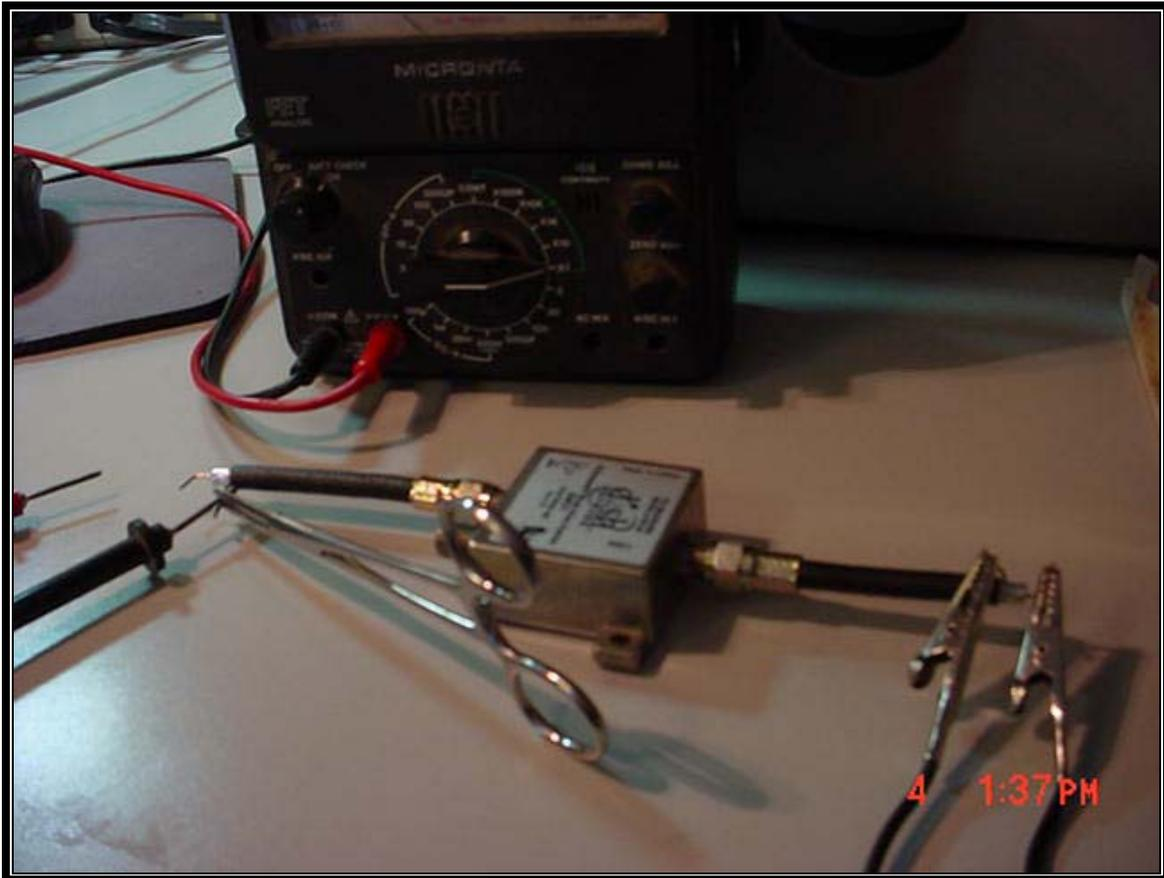
With a positive meter reading you can test each switch to check if the switch is good or bad before installation or after a problem has occurred.
