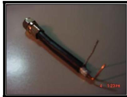
Preparation cut two small pieces of rg6 cable around 4-6 inch's, trim back both ends with your wire strippers to about 1"inch. Roll the exposed strands of wire together into a string making each about  $\frac{3}{4}$ " long. I trim the cooper center wire and with my needle nose piles turn the ends up 90 degrees.
