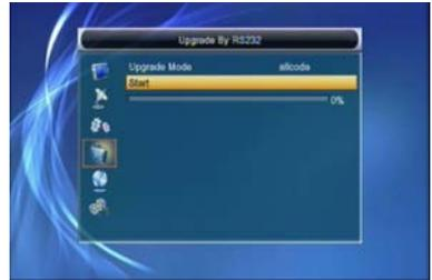
2 Connect master receiver to slave receiver via serial interface. Enter “Upgrade By RS232” menu receiver and press [Volume
